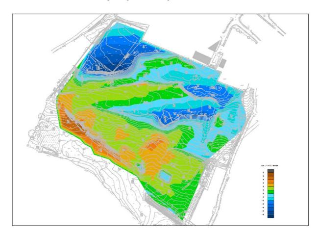
Volumetric surveys can also be applied to stockpiles, quarries, landfill, open excavations and backfilled areas to accurately quantify the cut and fill volumes.
